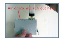
Push the ink into the cartridge from the nozzle, with a syringe that is cut a 2mm hole.
