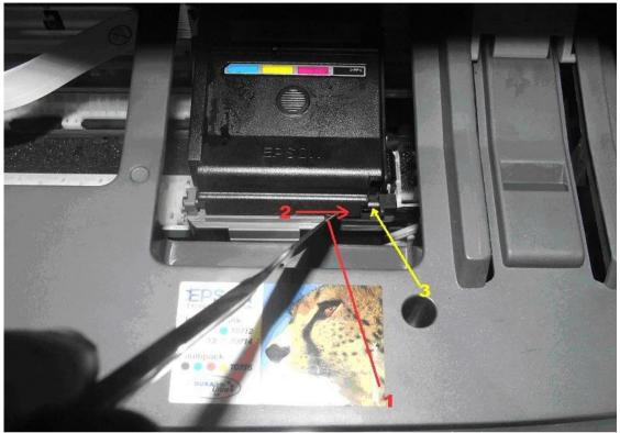
Number 1... There is a gap here. You need to put a thin object like a screwdriver or table knife into the slot. Number 2... Once the screwdriver/knife is in the gap, twist to the right and you will see the small plastic bit move.
