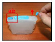
4. Pull out the rubber seals from the Ink Filling Hole.
