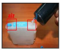
5. Insert the syringe into the Ink Filling Hole.
