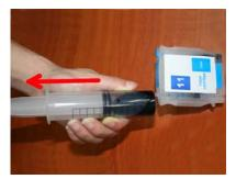
7. Draw the plunger upward (about 20ml space), then loosen it.
