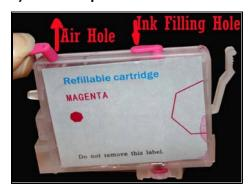
Please seal the refilling hole with plugs and open the air hole when you print.
