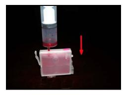
Then loose the plunger. The air pressure will push lnk flow into the cartridge naturally.
