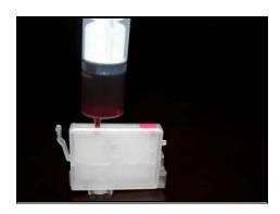
Insert the syringe into Ink filling hole; Please make sure that the syringe fits well the Ink filling hole; Otherwise, you couldn't vacuum the cartridge.
