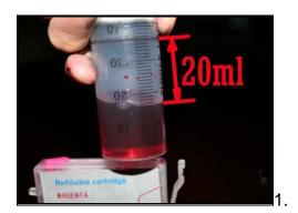
Pull up the plunger for about 20ml to vacuum the cartridge;
