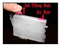
Pull out the rubber plug from Ink filling hole;
