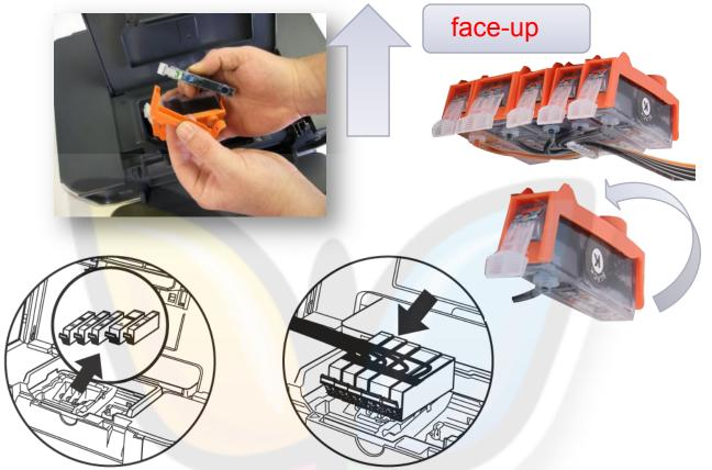
4. In the one motion turn the set of cartridges over and install all together into their respective houses in the printer head housing unit. You'll know each cartridge is in its <u>correct place</u> when you've heard it click in, just as if you were installing a Canon original cartridge.
