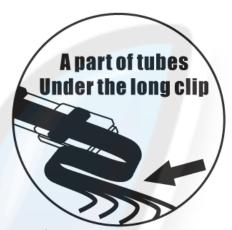
2. The purpose of the ink pipeline holder is to fix a section of the pipeline to the frame so that the ink pipeline will not be damaged nor blocked by the movement of the printer head back and forth.
