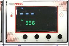
Press OB button, the temp III light is on. Select with arrows the temperature according to different transfer material (Normally 180°C~200°C) SV: Set temperature PV: Current temperature
