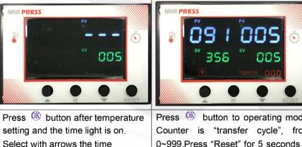
Select with arrows the time according to different transfer material. SV: Set temperature PV: Current temperature
