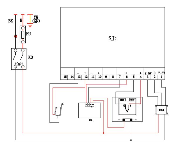
$K_0$ : Power Switch FU:Fuse SJ: Digital Controller R1:Relay
