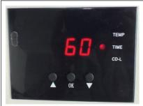
Press button after the temperature setting and the time light is ON.
