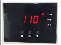
Press  $\bigcirc$  button, the temp  $\bigcirc$  light is ON. Press Up " $\triangle$ " or Down " $\nabla$ " button to set temperature according to different transfer material. (Normally  $180^{\circ}$ C~200 $^{\circ}$ C)
