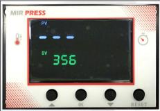
Press button, the temp light is on. Select with arrows the temperature according to different transfer material (Normally 180°C ~ 200°C)
