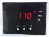
Press button, the temp light is on. Select with arrows the temperature according to different transfer material (Normally 180°C~200°C)
