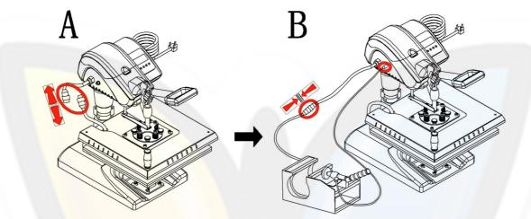
Disconnect the heat platen wire. Connect the mug press, one socket is power socket The other one is limit switch socket
