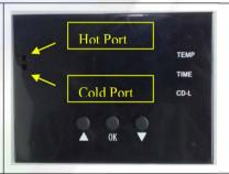
Note: There are two small port in front side of the digital display. If the real temperature is lower than digital controller shown, you can adjust the "hot port"; Clockwise to raise temperature; anticlockwise to reduce temperature.
