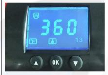
Press button, the temp light is on. Select with arrows the temperature according to different transfer material (such as 360°F).
