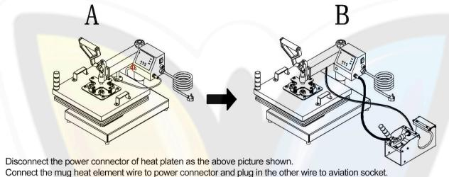
Connect the mug heat element wire to power connector and plug in the other wire to aviation socket.
