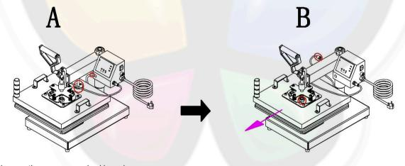
Please loosen the screws marked in red. Disconnect the power connector as the above picture shown.
