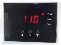
Press button, the temp light is on. Select with arrows the temperature according to different transfer material (Normally 180°~200°C)
