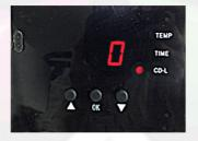
Press ok button after time setting; the display shows the temperature starts to rise. "CD-L" shows the time counting down during your transfer.
