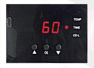
Press ok button after the temperature setting and the time light is ON. Press Up "△" or Down "∇" button to set time according to different transfer material.
