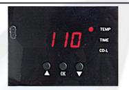
Press ok button, the temp [iii] light is ON. Press Up "△" or Down "▽" button to set temperature according to different transfer material. (Normally 180°C~200°C) Note: Temperature will be shown on the controller only after it reached to 100°C, it's normal that there is no temperature shows right after the setting.
