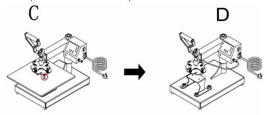
Remove the heat platen and under plate. Install the heat element as the above picture shown.
