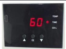
Press button after temperature setting and the time light is on. Select with arrows the time according to different transfer material.
