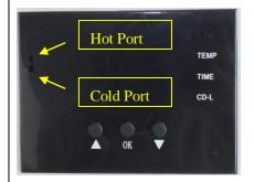
Note: There are two small port in front side of the digital display. If the real temperature is lower than digital controller shown, you can adjust the "hot port"; Clockwise to raise temperature; anticlockwise to reduce temperature.
