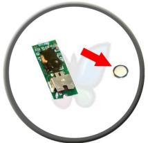
**Step 4.** When the battery has been removed, remember to keep it safe or make a note of the model number on the back so you can find the correct replacement. The battery model number is 377.
