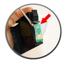
**Step 2.** If you wish to change the battery, use a small screwdriver to prize off the top or bottom of the chipset from the cartridge.
