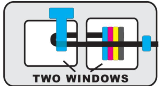
Looking into the printer from above, install the support clip(s) as shown. The one on the left (in the photos below) is called a *T-bar clip* and the one on the right is called a *square clip*. We have attached some photos below of various printers. Some printers use a T-bar clip, some a square clip and some printers use both.
