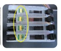
3. Installing the chip missing angle to the lack of angle and Install the chip Back to cartridge. Use the same ways to install all chips
