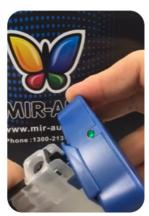
6. Use chip reseter to reset the original chipset, when light turns to green From red is ready to use.
