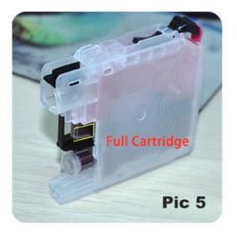
5) Inside each cartridge is a float that is Responsible for ink availability inside Cartridge, Before cartridge installation in Printer make sure the float is in Position Of Full cartridge (Pic 5).
